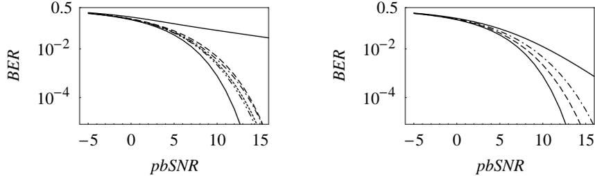
Left: **Figure 1a.** Bit error rate  $BER(N)$  plotted against per bit signal to noise ratio  $pbSNR$  in the case of coherent chaotic logistic spreading for spreading factors  $N = 1$  (upper solid),  $N = 2$  (dashed),  $N = 3$  (dot dashed),  $N = 4$  (dotted),  $N = 5$  (dot dot dashed) and lower bound (lower solid).
