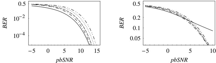
Left: **Figure 2a.** Comparison of  $BER(N)$  for the coherent and non-coherent lower bound, plotted against  $pbSNR$ . The solid curve applies to all spreading factors in the coherent case. In the non-coherent case, the lower bound curves are given for  $N = 1$  (dot dashed),  $N = 2$  (dashed),  $N = 5$  (dotted) and  $N = 10$  (dot dot dashed).
