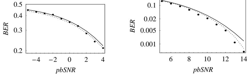
**Figure 3.** Bit error rates of the correlation decoder (solid) and simulated bit error rates of the optimal decoder based on 5000 samples (points) plotted against per bit signal to noise ratio  $pbSNR$  (left:  $-5 \leq pbSNR \leq 4$ , right:  $5 \leq pbSNR \leq 14$ ,) in the case of non-coherent logistic spreading with spreading factor  $N = 5$ . Dotted line indicates the boundary of a critical region with a significance level 0.05.
