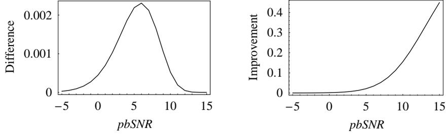
Left: **Figure 4a.** The difference between exact bit error rates of the optimal decoder and the correlation decoder plotted against per bit signal to noise ratio  $pbSNR$  in the case of non-coherent balanced binary spreading with spreading factor  $N = 2$ .
